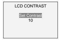
Press ENTER to modify the contrast. Select a value from 0 to 25, 25 producing the most contrast.
